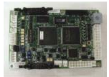
JSW original high-speed servo control board
